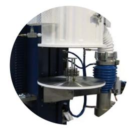
• It's a cold wall furnace, with cylindrical water cooled vessel and windows for visualisation;
