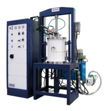
• This systems are designed for high temperature and high pressure consolidation of powder materials in oxidizing, high vacuum, inert or reducing atmosphere;
